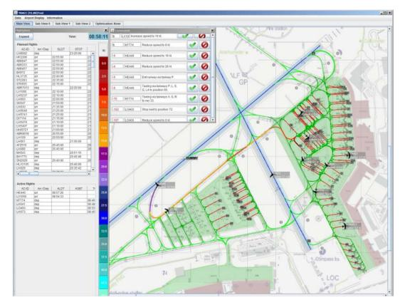
Figure 1. Main screen with view of the airport (map and node-link-system). Three sub screens for detailed views. Aircraft routes as colored lines (color depending on average speed). Expandable Tables with information about planned and active aircraft. Frame with actual controller commands.
