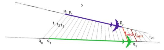
Figure 3. Time dependent minimum distance between two aircraft moving on vectors in space.
